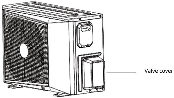
Remove protective caps from ends of valves. Align flared pipe end with each valve and tighten the flare nut as tightly as possible by hand. Using a spanner, grip the body of the valve. Do not grip the nut that seals the service valve. While firmly gripping the body of the valve, use a torque wrench to tighten the flare nut according to the correct torque values. Loosen the flaring nut slightly, then tighten again. Repeat steps for the remaining pipe.
