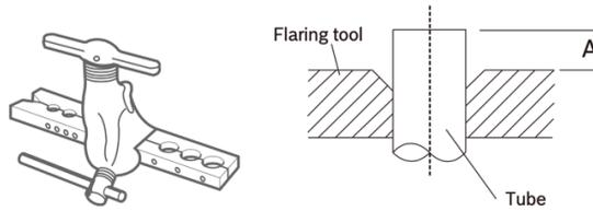
Clamp flare form on the end of the pipe. The end of the pipe must extend beyond the edge of the flare form in accordance with the dimensions shown in the table below. Place flaring tool onto the form. Turn the handle of the flaring tool clockwise until the pipe is fully flared. Remove the flaring tool and flare form, then inspect the end of the pipe for cracks and even flaring.
