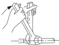
Tighten the flare nut as tightly as possible by hand. Using a spanner, grip the nut on the unit tubing. While firmly gripping the nut on the unit tubing, use a torque wrench to tighten the flare nut according to the torque values in the Torque Requirements table below. Loosen the flaring nut slightly, then tighten again.
